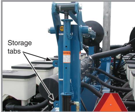
Row marker lockup installed
