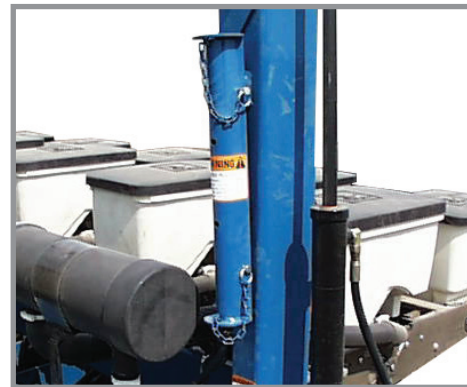
Row marker lockup in storage location
