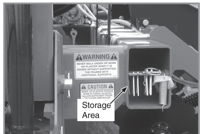
Spare chain link storage
