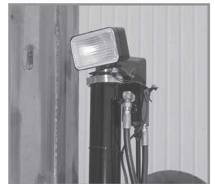
Auxiliary work lights
